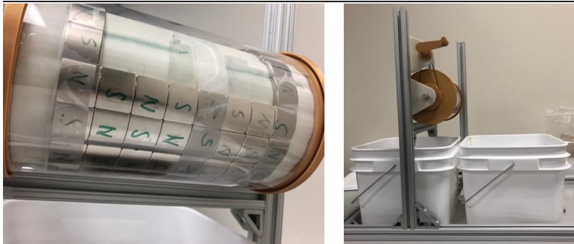
Figure 16. Magnetic Separator Experiment Apparatus.
