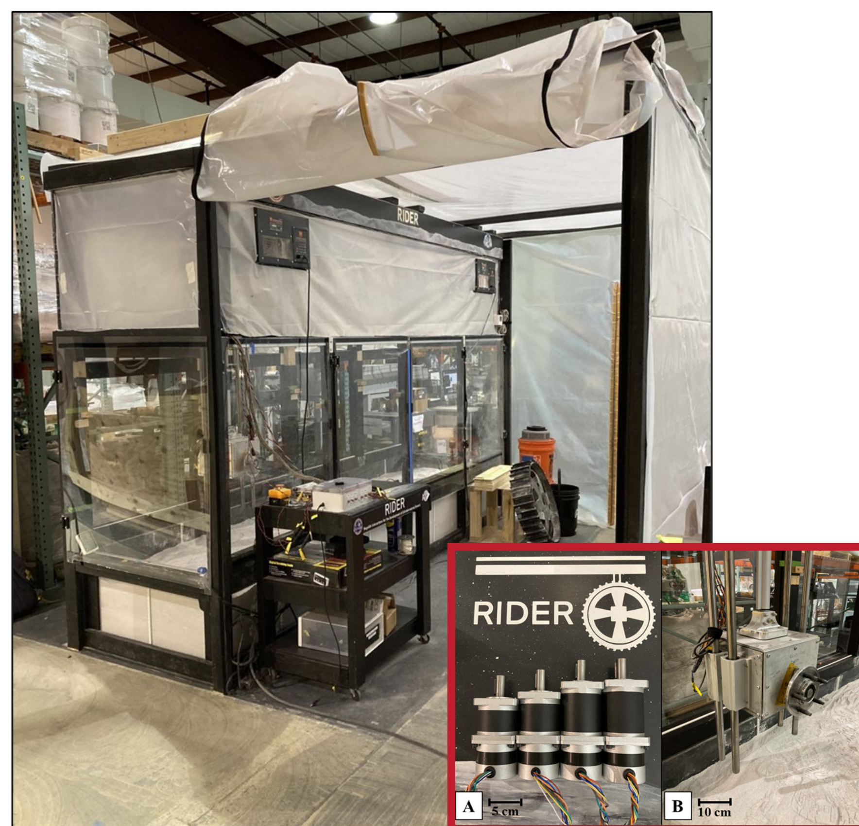
Figure 4. - Regolith Interactions for the Development of Extraterrestrial Rovers (RIDER) is housed at Exolith Lab. RIDER is a state-of-the-art, terramechanics testbed (3.8 m x 0.9 m x 0.5 m deep), designed to test wheel-regolith interactions. Inset: (A) 24 V DC brushless motor options for RIDER (10:1, 50:1, 100:1, 225:1), (B) motor-box and wheel hub assembly, attached to a linear actuator that serves as a gravity offloading system.
