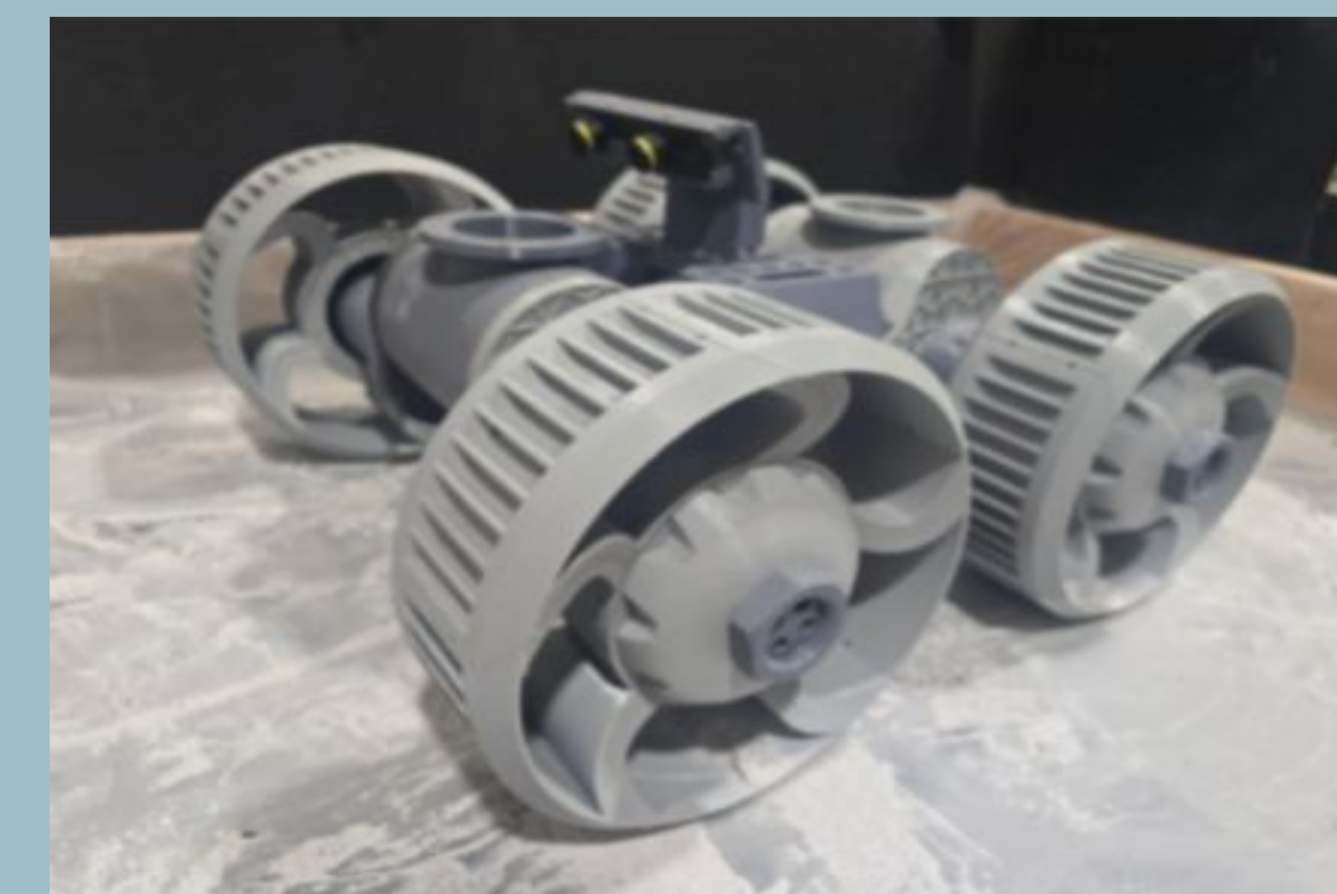
Figure 3. Cislune-built RE-RASSOR prototype advancing open-source, low-cost lunar excavation technology. A new unit is being rebuilt to document the full assembly supporting reproducibility and future design improvements.
