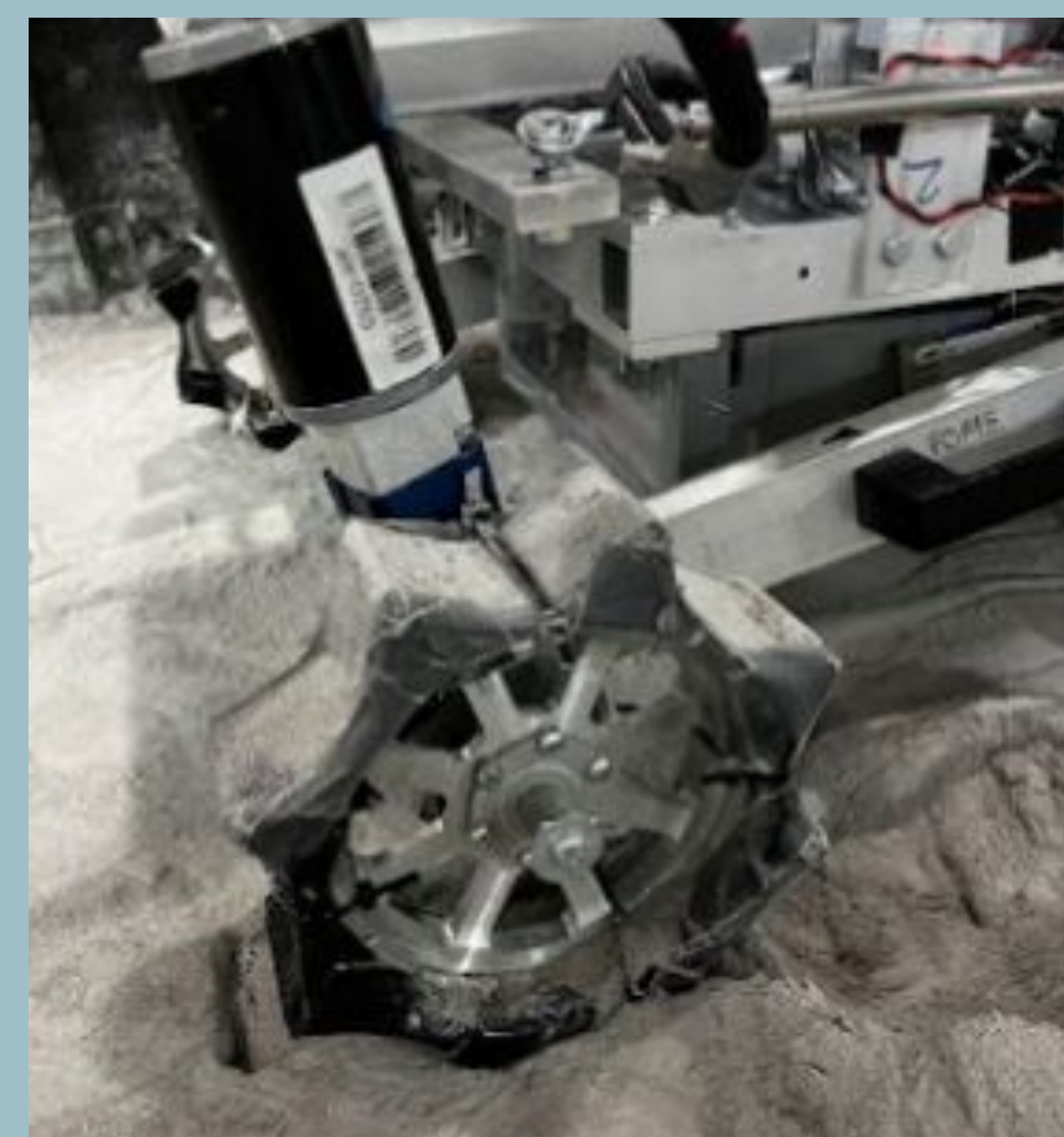
Figure 2. GRASP wheel prototypes evaluated using the RIDER testing system. The upper image shows the fourth wheel undergoing active testing, while the lower image presents three previously tested designs used to collect data on traction, sinkage, slip, and other performance metrics for comparative analysis.
