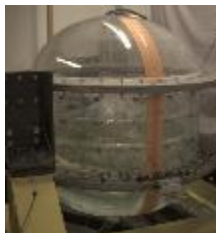
1/5 scale upper-stage LH2 and LOX tanks under test at ASAP Lab
